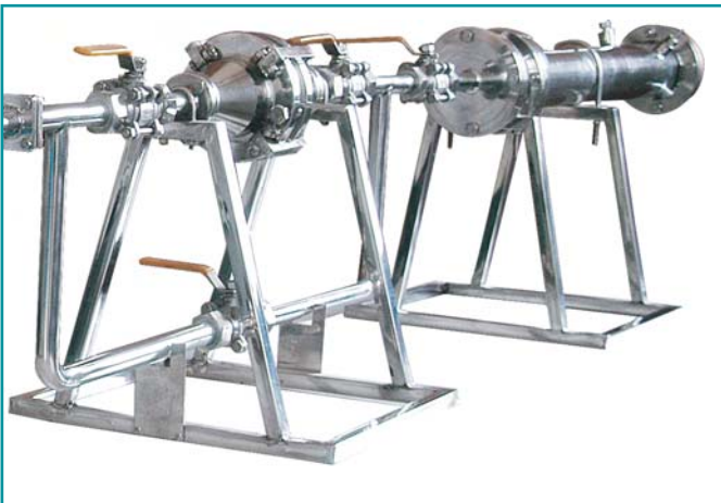
Compressed Air Suspended Oil Testing equipment-Drawing Samples
